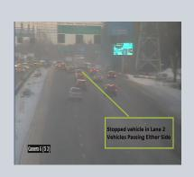
ClearWay detects a stopped vehicle. The radar software generates an alarm and directs the camera to the incident. The poor weather reduces the image quality, however, the radar still detects the event.
