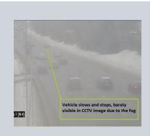
The radar detects a stopped vehicle in thick fog. The camera is unable to provide a clear picture due to the fog however, ClearWay's performance is unaffected.
