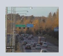
Radar detects a stopped vehicle during heavy traffic. The nearest camera is redirected to provide a visual giving the operator more information about the event
